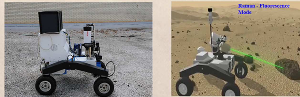
(a) Laser beam in (a) pointed to the surface target sample (b) future applications of remote Raman on a planetary surface rover.
